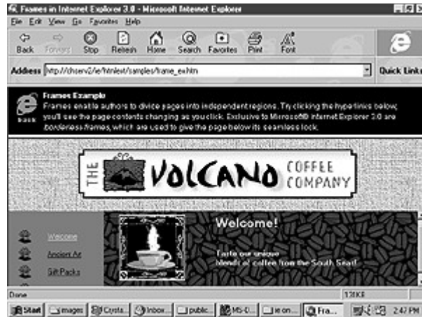
• Figure 4 Floating Frames: Insert a Web page into a Web Page as easily as embedding a graphic.
